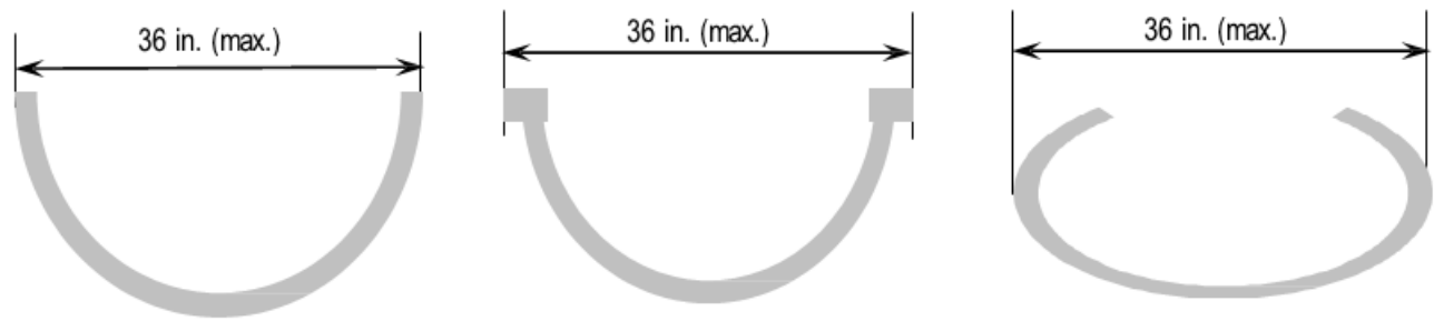
Figure 2.1 – Definition of Maximum Width Measurement (Not to Scale)
